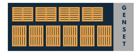
Can be loaded up in 1 layer with 9 VMF industrial pallets with a dimension of 1000x1200 mm (for goods that do not protrude beyond the outline of the pallet).
