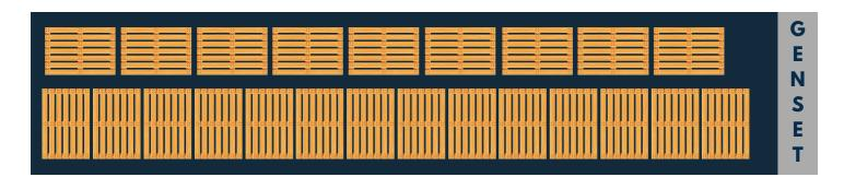
Can be loaded up in 1 layer with 20-21 VMF industrial pallets with a dimension of 1000x1200 mm (for goods that do not protrude beyond the outline of the pallet).
